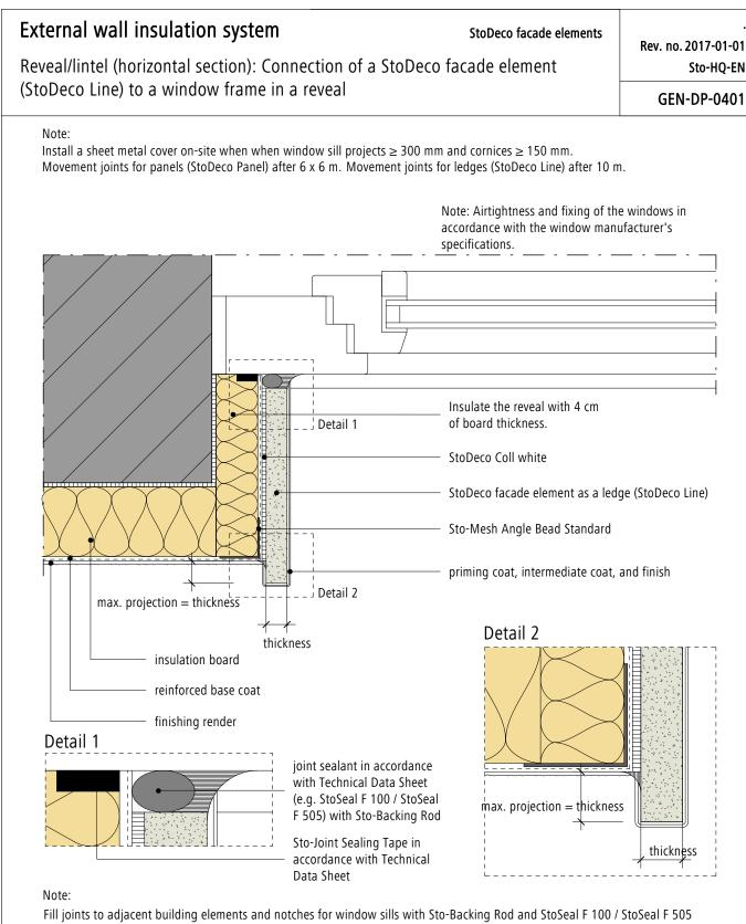
in accordance with IVD Data Sheet no. 9 or with Sto-Joint Sealing Tape in accordance with the Technical Data Sheet. Form connection joints as fillet.
